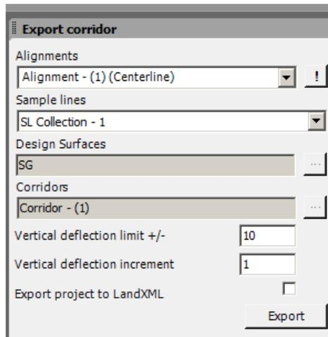
Figure 4: Civil 3D Screen with ExportCorridor Plug-in Panel
